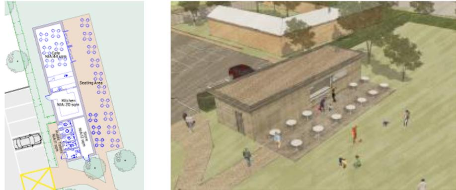
This could be done using modular construction, made in a factory and transported to the site. Figure 3 is an example. This could cost substantially less, although the overall cost may not be much different to new building of lower specification, matching that of the modular form.
